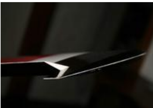
Check for enough movement Sand the wipers if not enough
